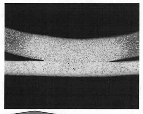
Photograph above of THERMAFIN fintube cross section (magnified 46 times) shows how the high frequency forge-welding process provides complete and permanent bonding of fin to tube, as evidenced by the grain growth across the joint.
